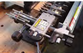
Creative stops. Omnijig stops, used to position the templates, were calibrated correctly for straight-from-the-box use, but can be fine-tuned.
